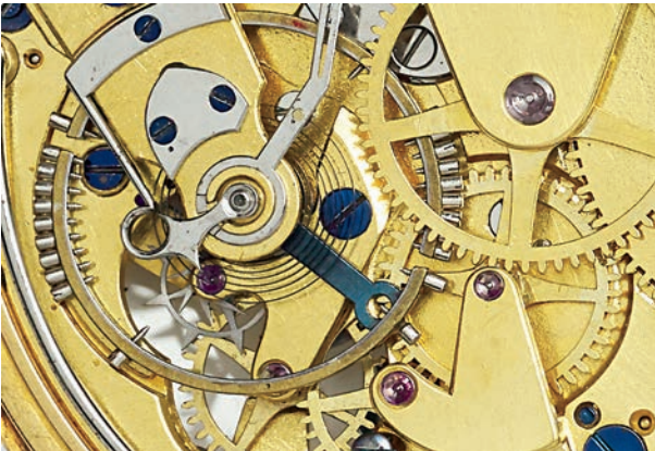
Detail of double Duplex escapement
